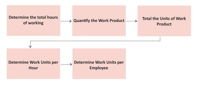
Fig. 2.9 Steps to Calculate Manpower Estimation for Production
