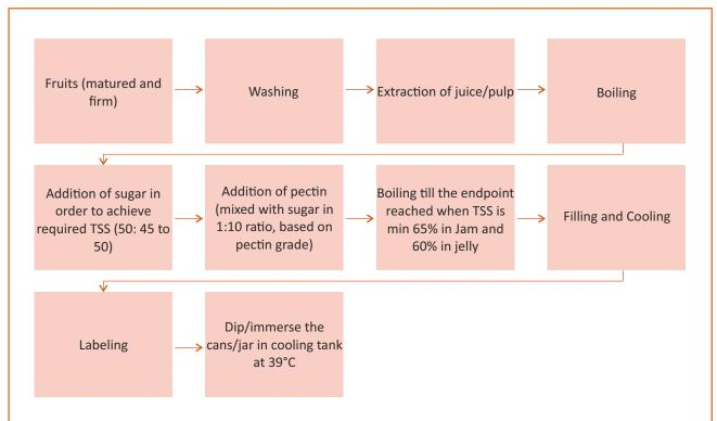
Fig.5.12 Process flowchart for preparation of jam
