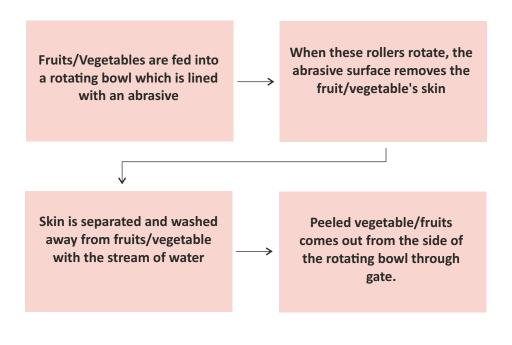
Fig. 3.14 Process of Peeling Machine
