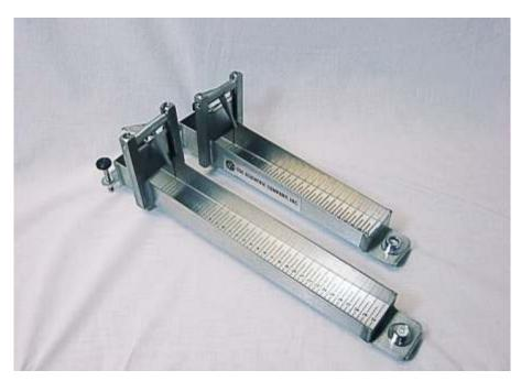
Fig 6.4 Bostwick Consistometer (Source: https://www.cscscientific.com/consistometer/bostwick-consistometer)
