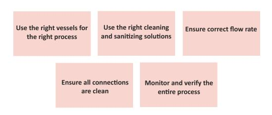
Fig 3.32 Tips for conducting an effective CIP process
